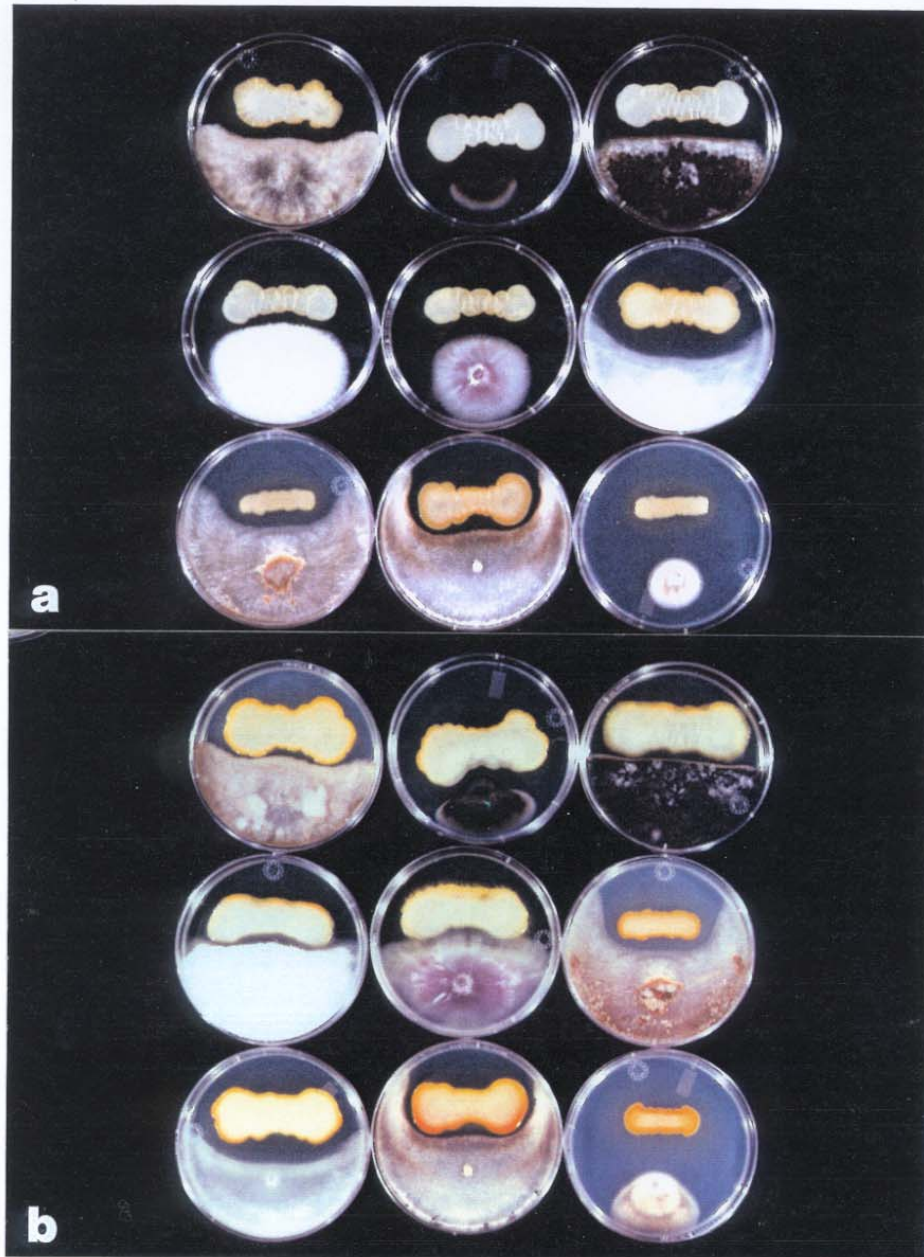
Figure 2. Photographs of the same test panel of fungi to show the effect of time on the rating assigned. (a) taken after 6 days, and (b) taken after 11 days. Note that the right plate in the middle row and the left plate in the bottom row of photograph (a) have exchanged places in (b)
